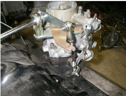
110 or Two Carb Linkage Kit used with manual choke
