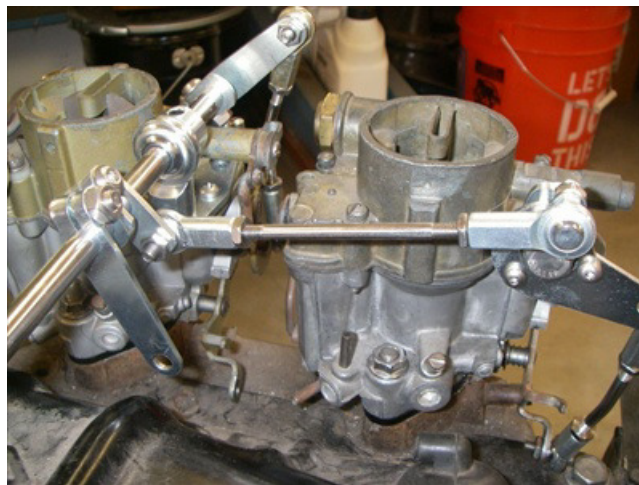
NEW – 140hp Non-Progressive Linkage. All 4 Carbs move as one - Left Side Shown. Appearance is just like the 1965 140hp Linkage. Will work on 1966-69 140hp with the Choke Lock-outs removed.
