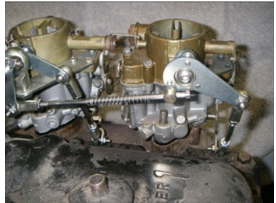
1966-69 140hp Right Side. Using Choke Lock-Outs.
