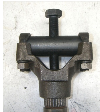
Yoke Puller installed for use On 1960-64 Axle
