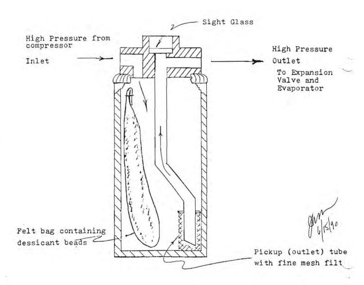
As for the desiccant, it was found to consist of a varied assortment of brittle glass-like beads of BB size contained within a 1/8-inch thick felt bag which was, rather crudely, merely folded over and stapled to close. These beads were brittle and shattered like glass when squeezed with pliers. They were black in color. When baked in a 300 degree F oven for an hour they did not change color (i.e., from pink to blue--or whatever) so it is assumed they are not of a "normal" desiccant composition.
