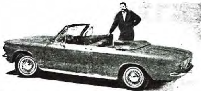
MONZA SPYDER version of the rear-engined Chevrolet Corvair is shown here with the optional centre-lock wire wheels.
