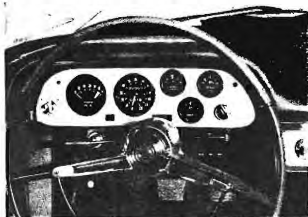
FACIA PANEL of the Monza Spyder carries a full set of instruments; a red sector on the tachometer starts at 5,000 r.p.m., the boost gauge reads up to 30 in. hg. (approx. 15 lb./sq. in.) above atmospheric and a thermometer scale for fan-cooled cylinder heads reads to 600°F.
