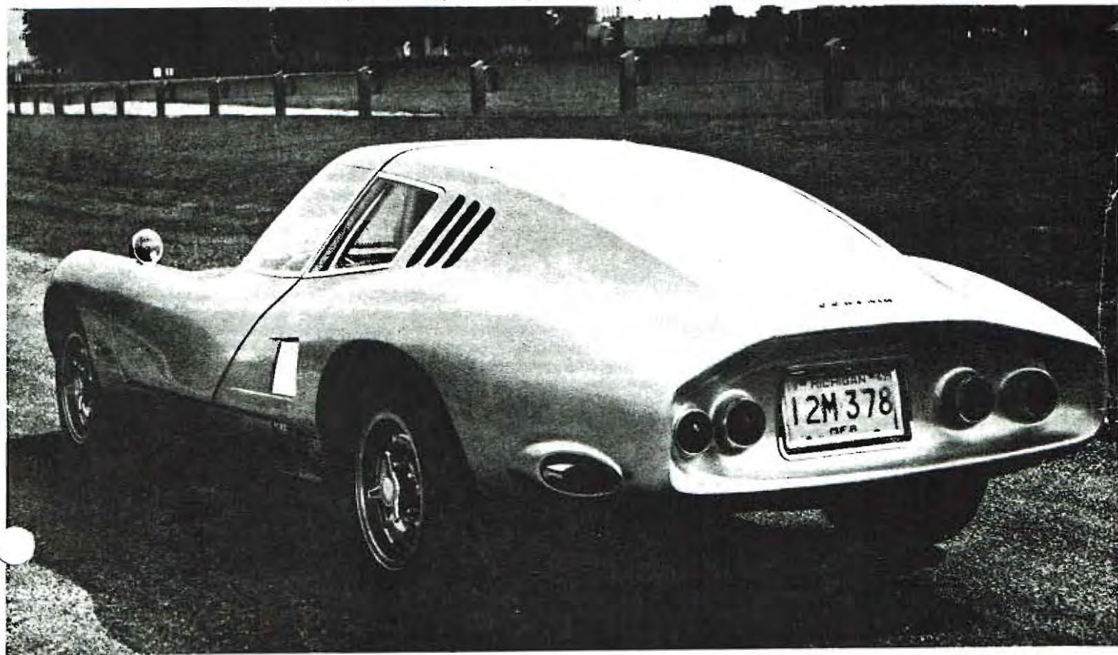
Forward visibility is excellent; rear view (and ventilation) can be increased by opening louvered section of top.
