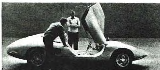
Cockpit entrance is gained by lifting canopy.
