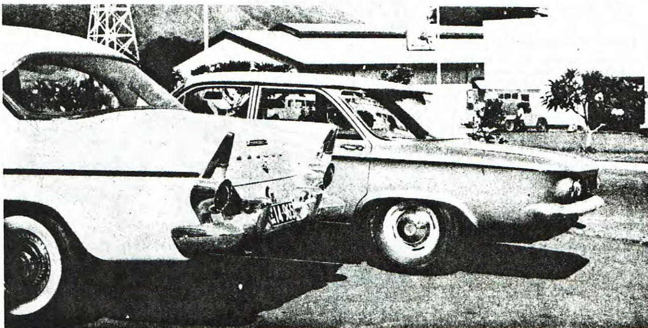
AIR-COOLED flat-six sits low in tail, with all accessories on top and easily accessible. Note "left-hand drive" sign near numberplate. BELOW: Corvair is 4ft. 3½in. high, looks tiny beside a Holden.
