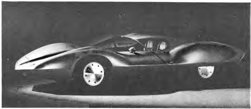
Astro I was a 1967 dream car powered by a highly modified OHC flat six. Tilt-up rear gave passenger entry and revealed powertrain.
