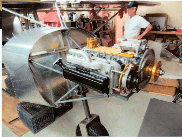
Right: Recently, Ron invited me and a couple of other neighbors over to help him lift the Corvair engine from the work bench to it's final resting place in the airplane. The engine as seen here weighs 213 pounds and will produce about 100 horsepower.
