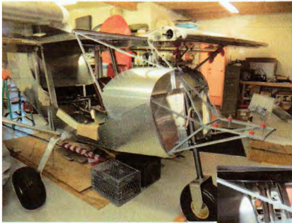
Left: .020 sheet aluminum is used to fabricate the skin of the Zenith CH-750. Ron is just finishing the last couple of pieces to complete the project. The motor mount is ready to receive it's new Corvair power plant. The engine will sit on the four red urethane bushings that can be seen here.
