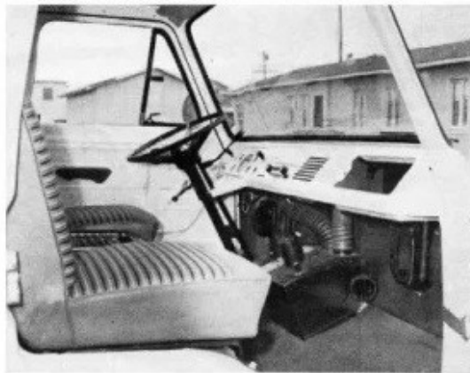
Ford's interior and ultra-tall windshield is not for people with acrophobia. Note safety wheel, exposed heater.
