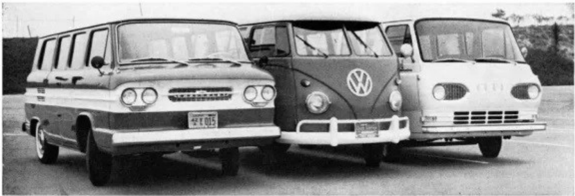
Ford, with front engine, is easiest to load from rear. Greenbrier and VW have step-ups over the engine.
