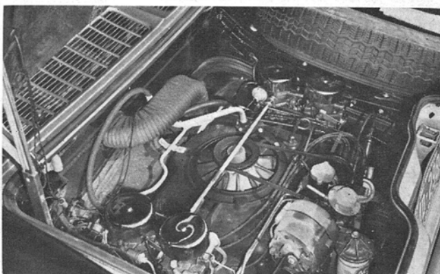
Miniature, chromed individual air cleaners replace umbrella-like unit in standard 4-carb Corvairs. Spare remains in back.
