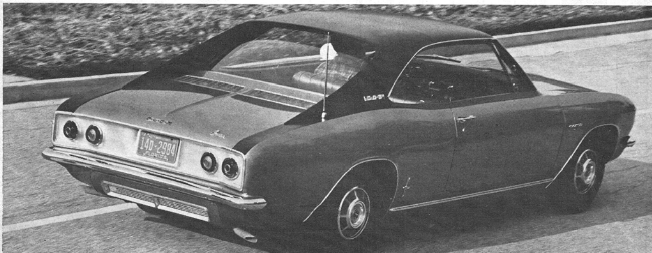
FIRST TEST CAR, SHOWN HERE, DID NOT HAVE OPTIONAL FITCH DUAL-EXHAUST SYSTEM, WHICH PROTRUDES THE PIPES DIRECTLY REARWARD.
