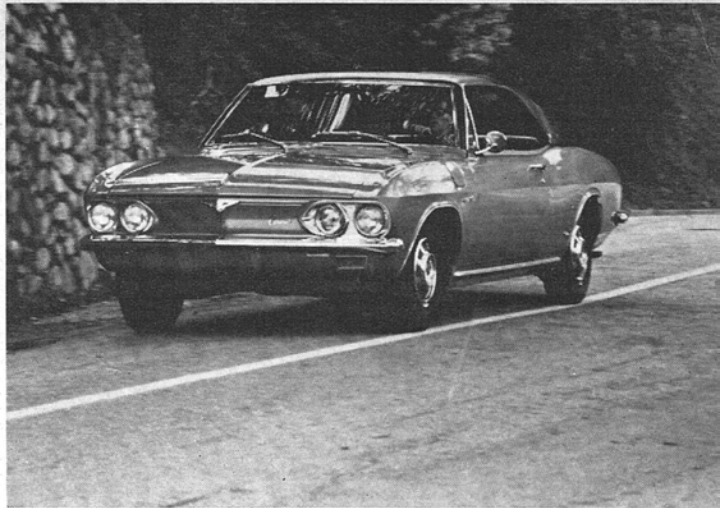
Unlike earlier models, an optional mesh covering the Sprint "grille" is not offered. Left high beam is Lucas "flame thrower."
