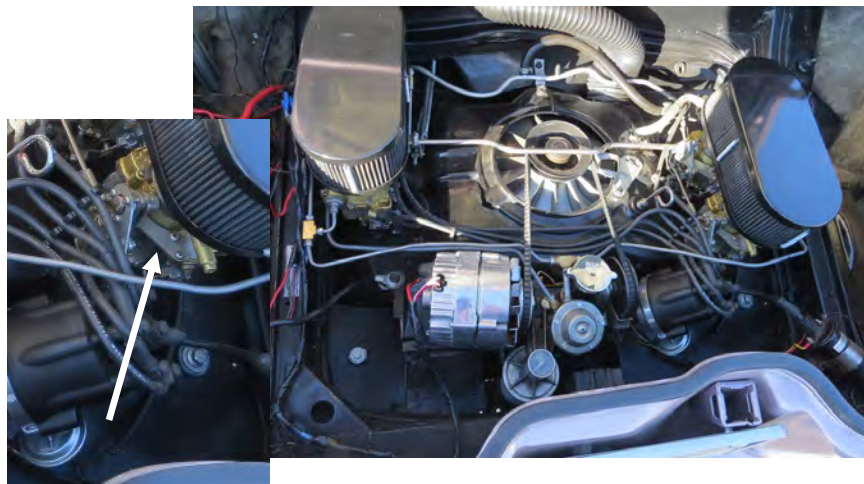
Below is Ron Bloom's 140 with a Seth Emerson Stinger distributor. A special kit is needed to achieve proper clearance.
