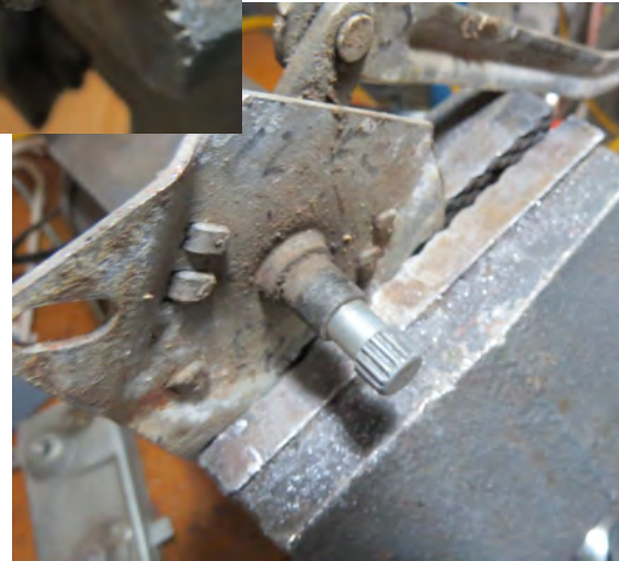
The old spline was removed from the door latch assembly with a hack saw (left) as well as the new spline from the window regulator (below).
