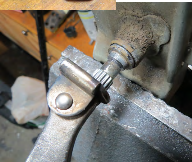
The new spline was clamped in place (left) and welded (above). Even though the weld is a bit large, there was no need to file it down since there was still plenty of clearance for the door handle to slid all the way on.
