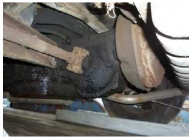
The Powerglide transmission (left) with the torque converter hanging out in space. On the Corvair it would be covered by a bell housing. On cars with a manual transmission, a round plate covers the hole where the bell house would have mounted (right).
