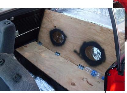
Even though Mike has spent months on his project thus far, there is still a lot of work to be done. The wood grain (non-telescoping) steering wheel brings a nice look to the car's interior (above). The back seat has been removed and replaced with plywood which Mike has prepared for stereo speakers (left). Lots of sound proofing material has been applied throughout the interior of the car.
