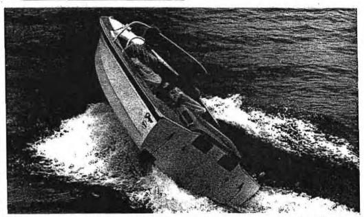
This type of quick maneuver will sometimes bury the inboard rail, so be careful. Hull seems to pivot around a point amidship, as the power unit is driving both forward, and lifting the stern at the same time. Cooling air is drawn in through side openings in the engine hatch cover. Hot air is ducted through the transom along with exhaust; engine compartment is pressurized.
